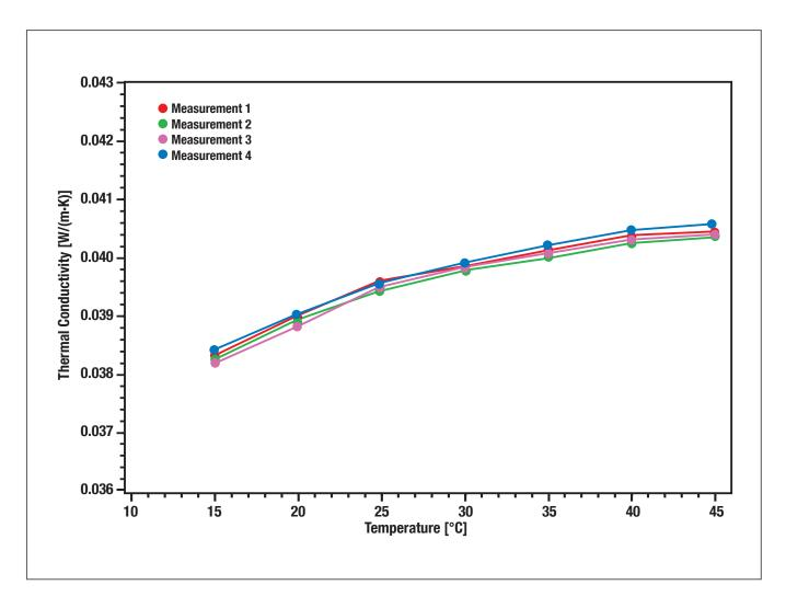
The present measurement clearly demonstrates the outstanding reproducibility of the LINSEIS HFM series. A reproducibility of 0.25% was achieved. The graph display four measurements of an Elastomer Foam
