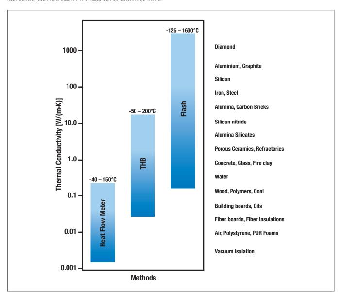
LINSEIS offers a complete range of thermal conductivity analyzers, ranging from Laser Flash and Xenon Flash Thermal constant Analyzers (small samples, liquids, powders, pasts, multilayer samples, broad measuring range and temperature) to Heat Flow Meters (Building and Insulation material) and a Transient Hot Bridge Analyzer (Solids, Liquids, Powders, Pasts and Gasses).
