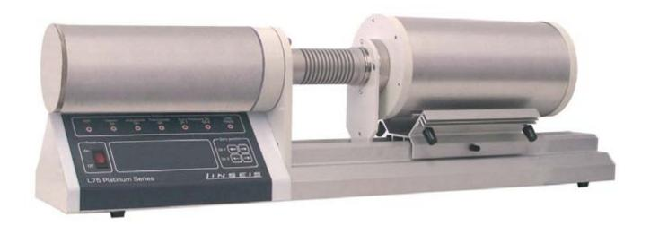
The newly developed DIL L76 Platinum Series is especially tailored to the needs of the glass and ceramic industries. High resolution and stability, wide measurement range, robust and compact design are only some of the advantages of the new, cost-effective system.
